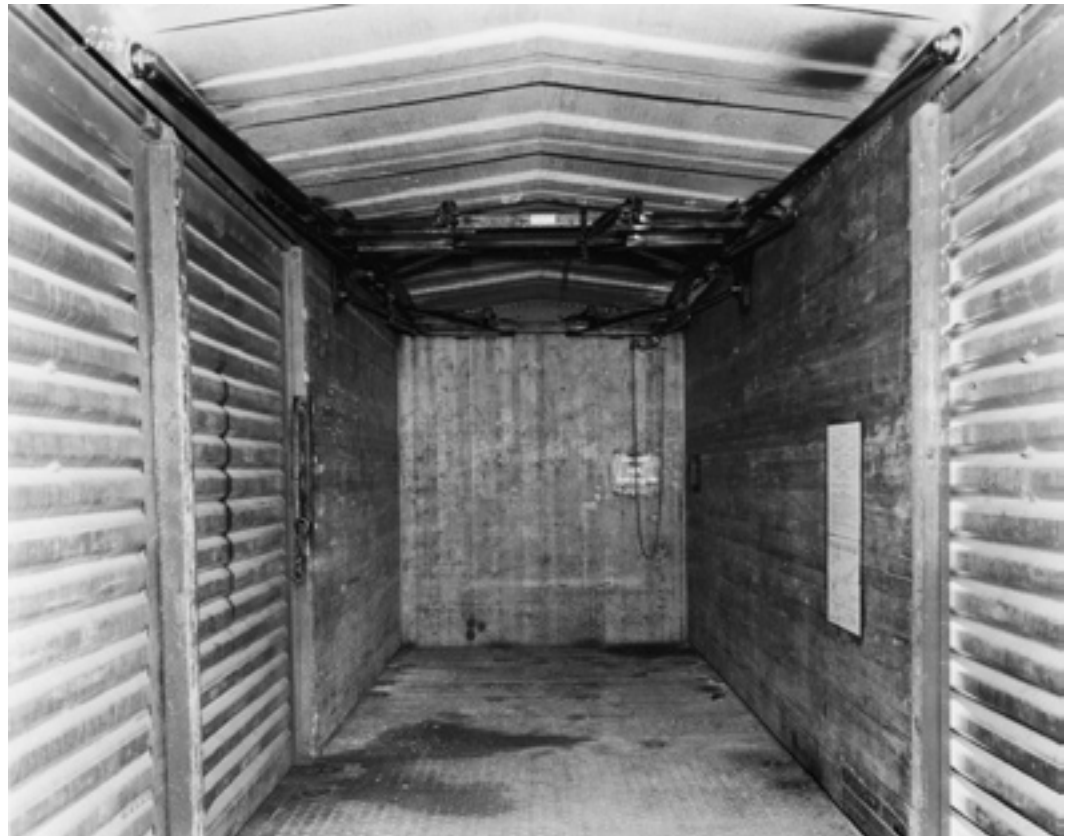
(Above) Type D Evans auto loading rack, in lowered position ready to receive vehicle, in Class A-50-12. Note perforated steel plate in door area.
