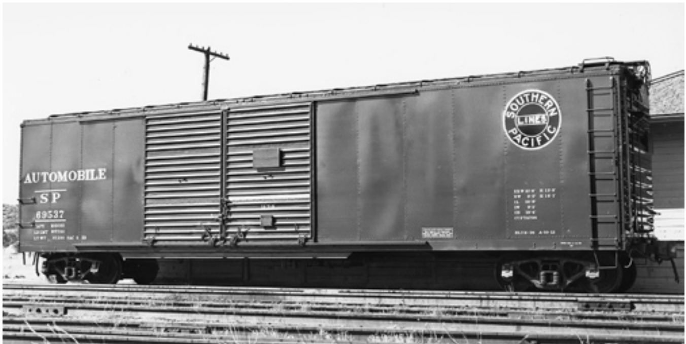
(Above) This photo dates from 1939, when the A-50-12 class was new. The single rivet rows attaching the side sheets are quite evident. (R.H. McFarland photo, Arnold Menke collection)
