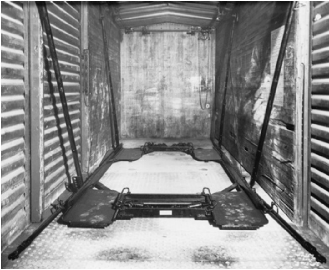
(Above) Type D Evans auto loading rack, in lowered position ready to receive vehicle, in Class A-50-12. Note perforated steel plate in door area.
