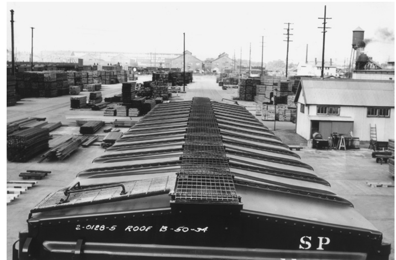
(Below) The diagonal-panel roof from SRECo is shown in this view at Car Shop No. 9 in the Sacramento General Shops complex. Also well shown is the U.S. Gypsum Company running board. This particular car is no. 110150. (both photos, Southern Pacific, SUL)
