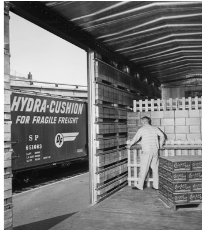
(Right, above) In January 1959, canned "Chicken of the Sea" tuna is being secured with Evans DF loader equipment in a B-50-47 car. (Southern Pacific photo, negative N-5365-1, Shasta Division Archives)
